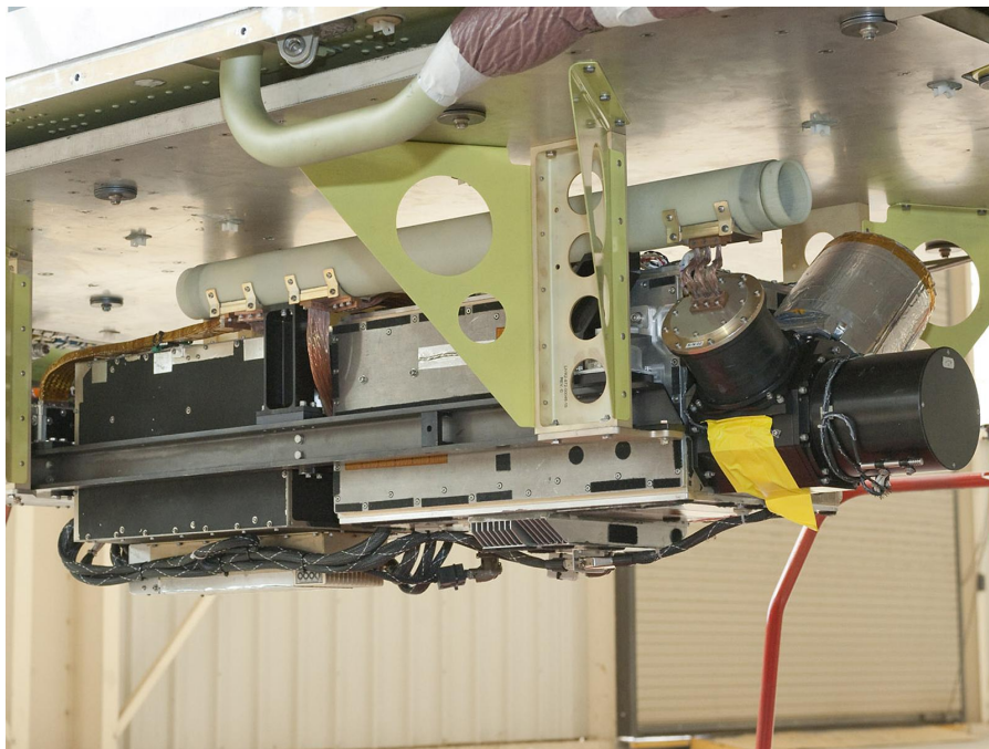
Figure 8: The S-HIS integrated to the Global Hawk with the heat straps (4 of 5 are visible) in place and connected to the rigid segment of the outside airflow tube.
