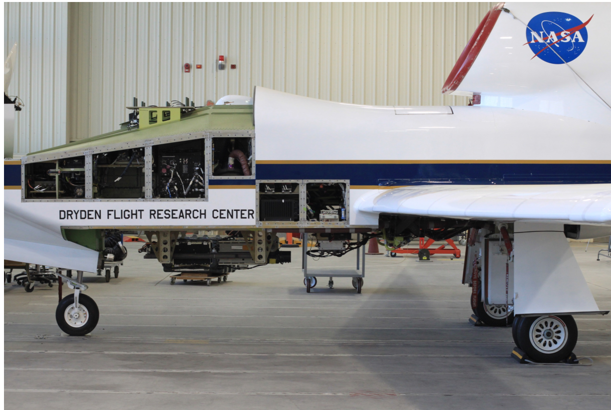
Figure 19: S-HIS mounted in Zone 25 on the NASA Global Hawk with fairing removed. The cooling tube is not installed in this photo.
