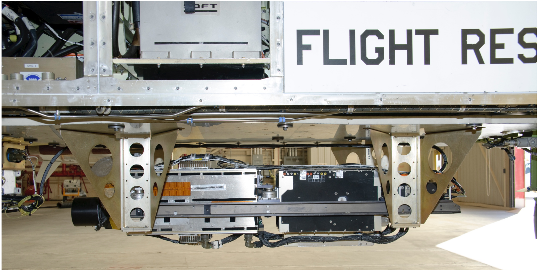
Figure 20: S-HIS in zone 25. The cooling tube is not installed in this photo.
