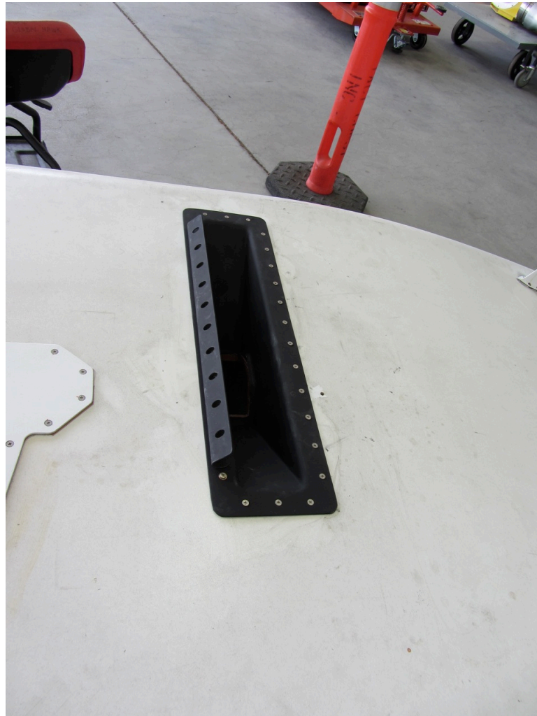
Figure 24: Close-up of S-HIS cross-track viewport and air dam (fairing removed from aircraft).
