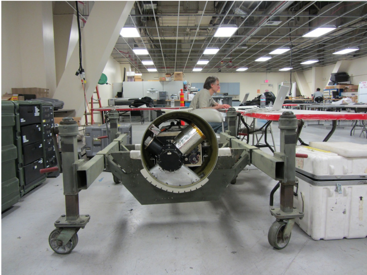
Figure 14: S-HIS mounted in ER-2 centerline pod.
