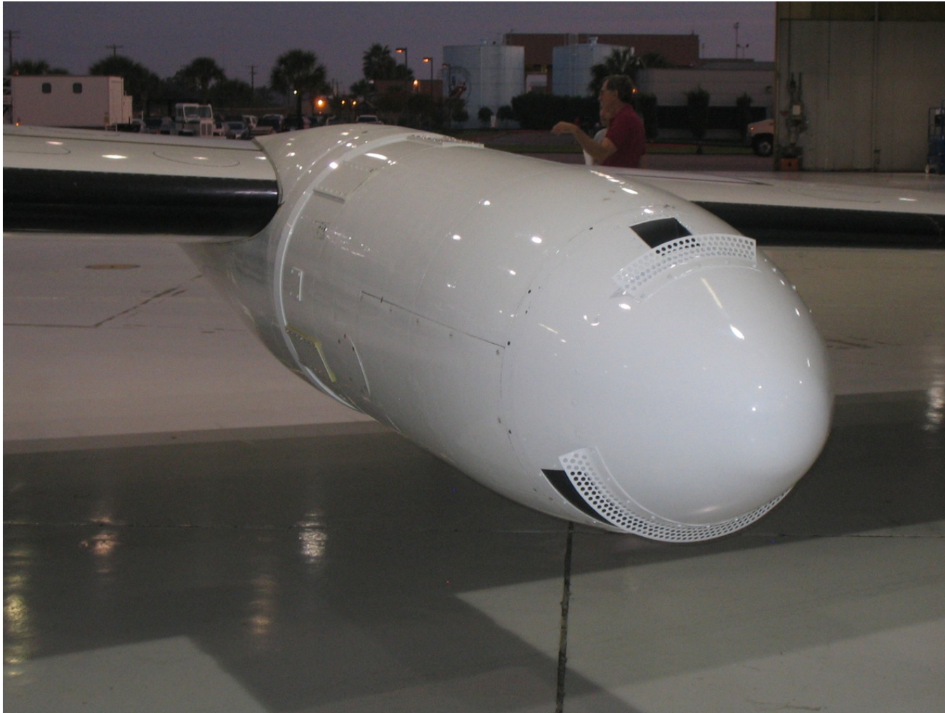
Figure 16: WB-57 Wing pod with S-HIS nose-cone installed. Zenith cross track ports and air dams are visible.
