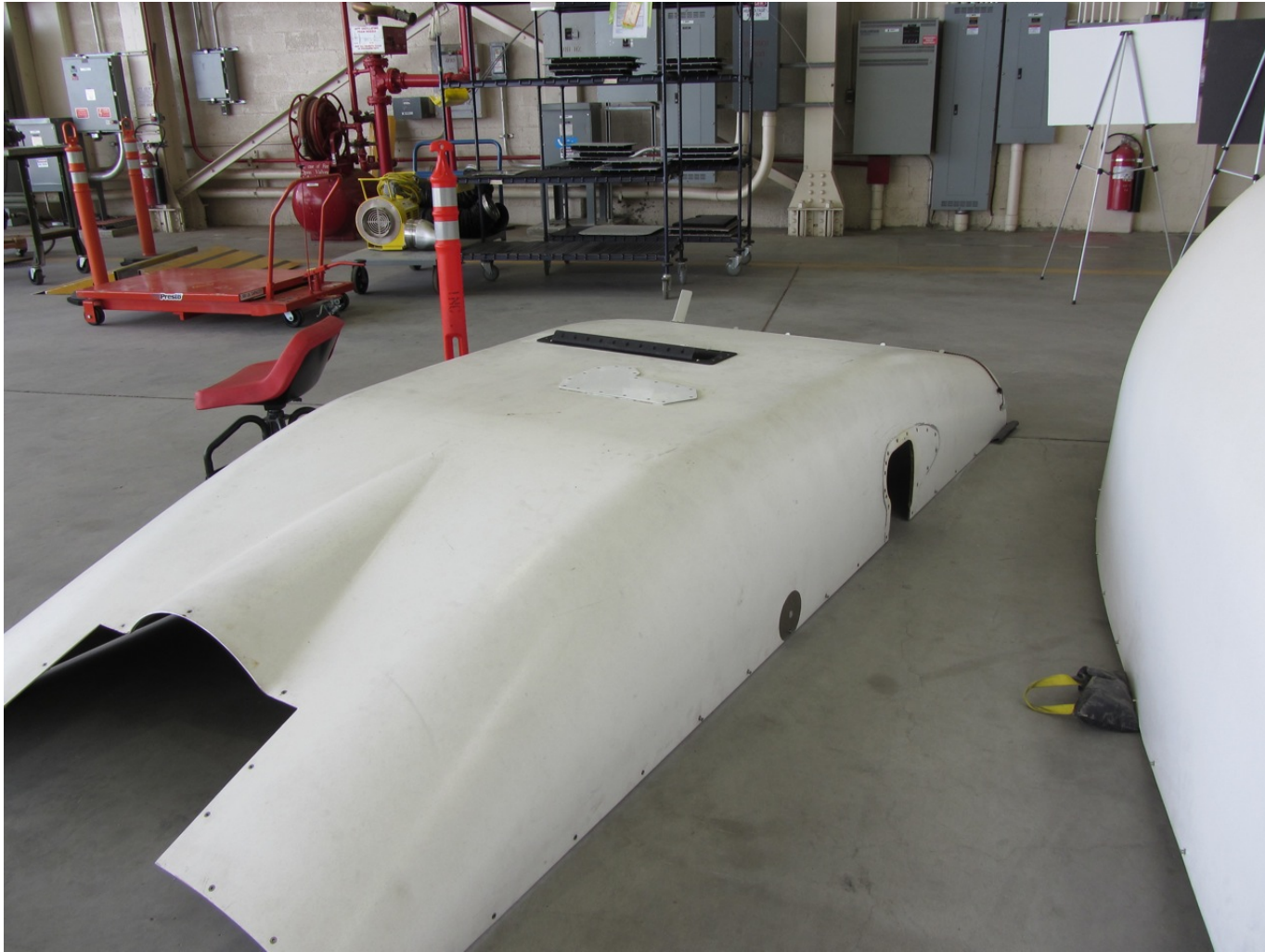
Figure 23: Global Hawk Zone 25 fairing with S-HIS cross-track viewing slot installed.
